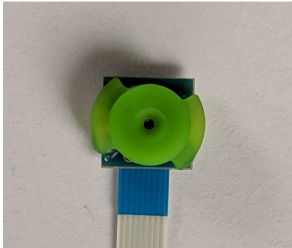
Figure 1. MOD_CH101-03-01 module with AH-10133-045045MR horn
