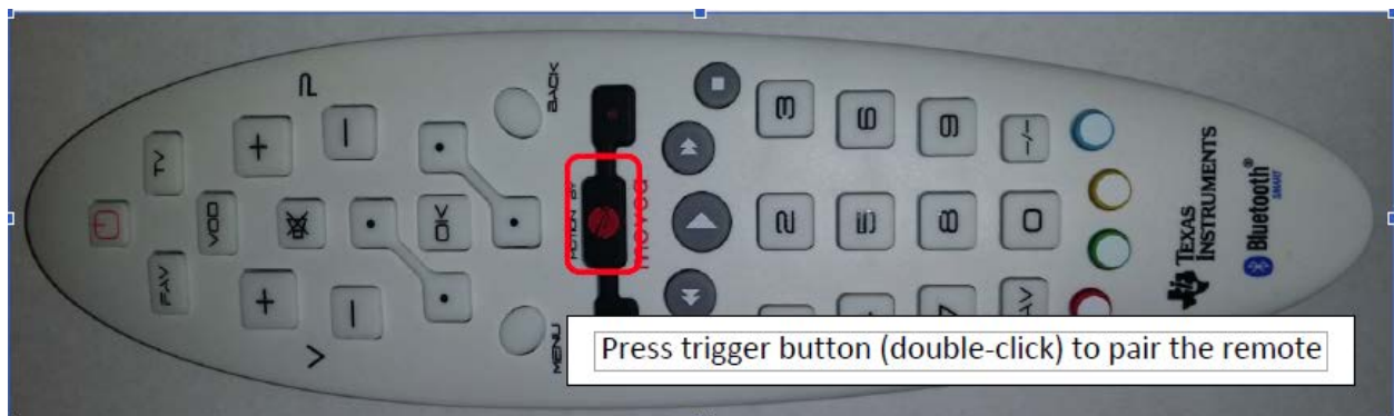
Figure 3: Trigger button to pair
