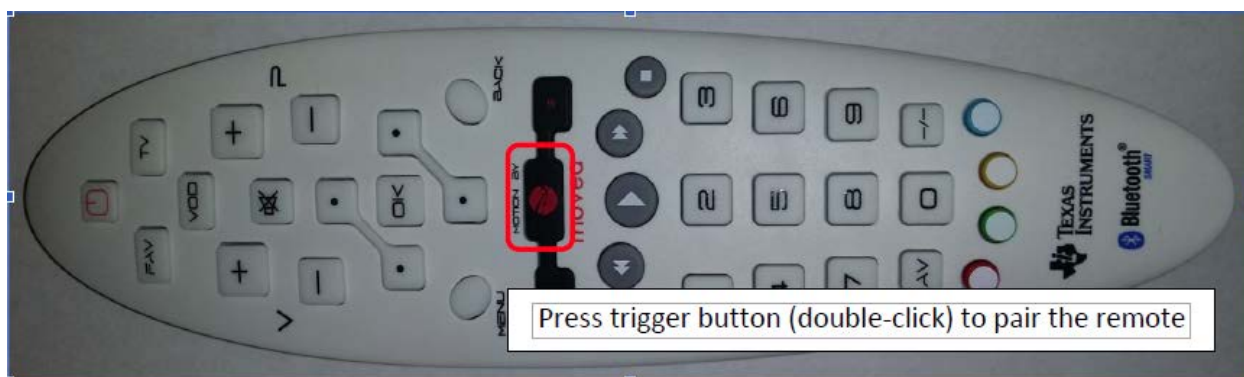
Figure 14: Trigger button to pair
