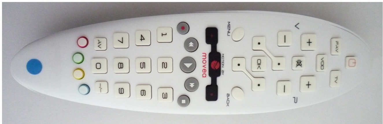
Figure 6: Blue button to pair
