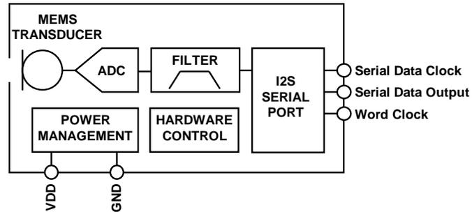
Figure 3. Typical I<sup>2</sup>S MEMS Microphone Block Diagram
