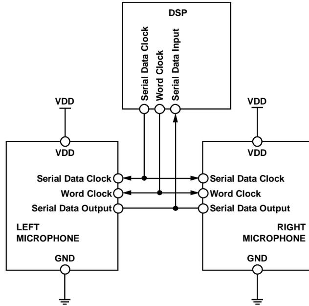
Figure 8. Stereo I<sup>2</sup>S microphone connection to a DSP
