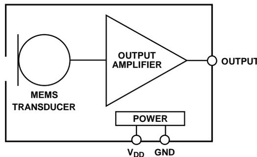
Figure 1. Typical Analog MEMS Microphone Block Diagram
