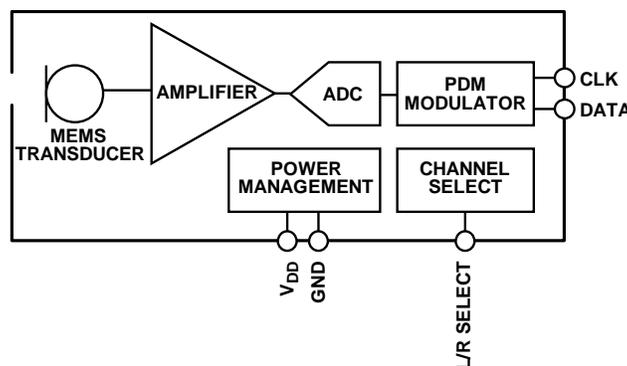
Figure 2. Typical PDM MEMS Microphone Block Diagram
