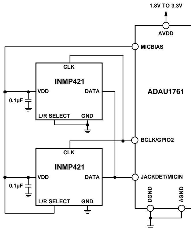
**Figure 1. Digital MEMS Microphone Connection to Audio Codec (Simplified Schematic: Power-Supply Decoupling and All Connections Not Shown)**
