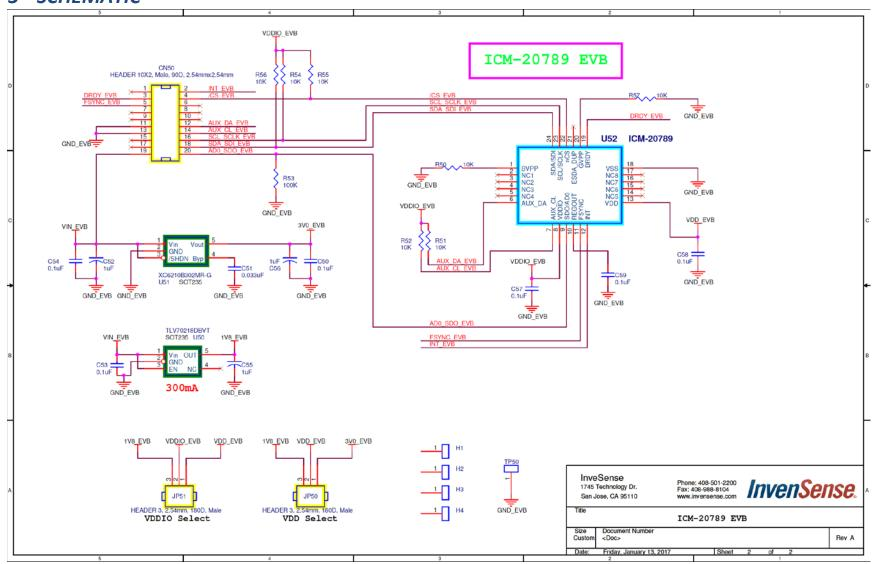
Figure 3. ICM-20789 EVB Circuit Schematic
