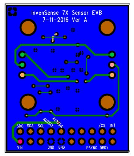
Figure 6. Bottom View of the ICM-20789 EVB Board Layout
