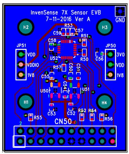
Figure 5. Top View of the ICM-20789 EVB Board Layout
