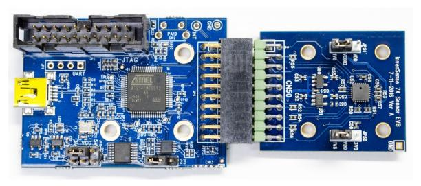
Figure 4. ICM-20789 EVB connected to the InvenSense ARM Controller Board
