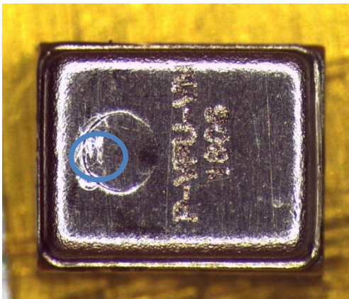
Closed vent hole
