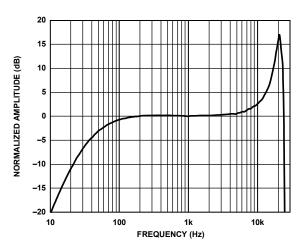
Figure 5. Typical Frequency Response (Measured)
