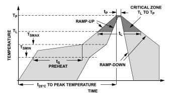
Figure 2. Recommended Soldering Profile Limits
