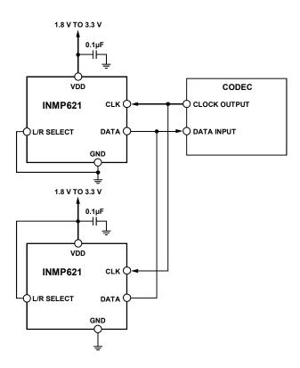
Figure 14. Stereo PDM Microphone Connection to Codec
