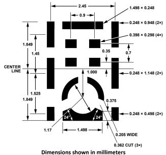
Figure 17. Suggested Solder Paste Stencil Pattern Layout
