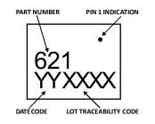
Figure 21. Package Marking Specification (Top View)
