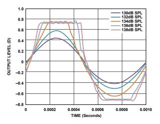
Figure 9. Clipping Characteristics
