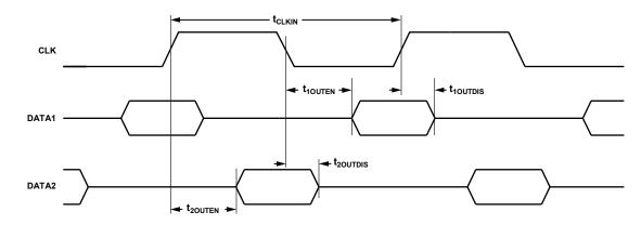
Figure 1. Pulse Density Modulated Output Timing
