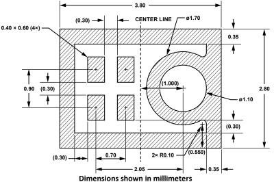
Figure 16. Recommended PCB Land Pattern Layout
