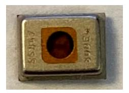
Figure 20: Top port of ICS-40800 with tape cover
