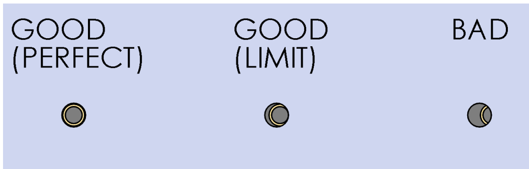
Figure 16. Examples of various degrees of CH101 port alignment with the Acoustic Interface, from perfect concentric alignment (left), maximum acceptable limit tangent alignment (middle), to bad occluded alignment (right).
