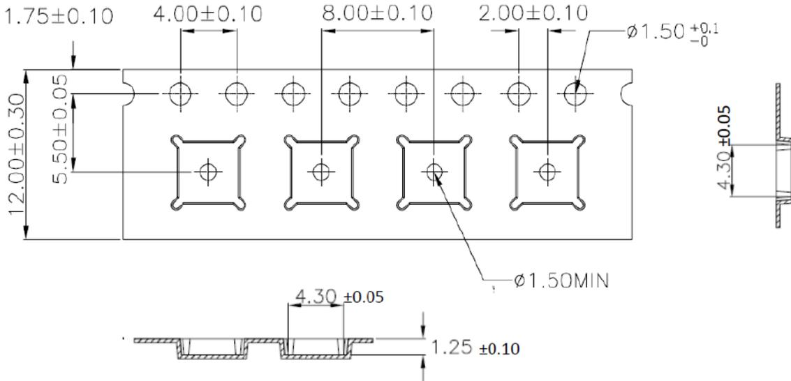
**Figure 15. 4 x 4 mm² Tape Dimensions**
