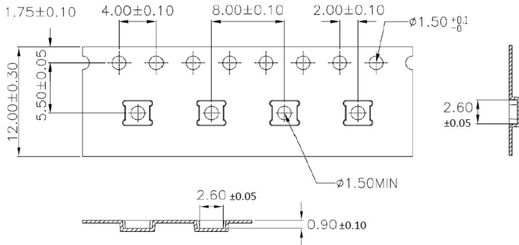
**Figure 18. 2.3 x 2.3 mm² Tape Dimensions**
