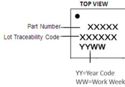
**Figure 13. 2.5 x 3 mm<sup>2</sup> Package Marking Specification**
