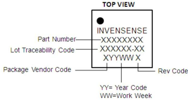
**Figure 8. 4 x 4 mm<sup>2</sup> Package Marking Specification**
