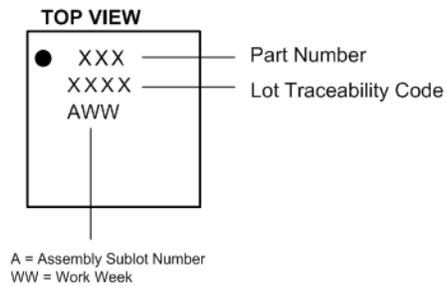
**Figure 11. 3 x 3 mm<sup>2</sup> Package Marking Specification (TYPE III)**
