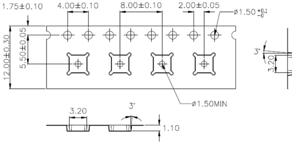
**Figure 16. 3 x 3 mm² Tape Dimensions (TYPE I) (for package height 0.9 mm and 1.0 mm)**
