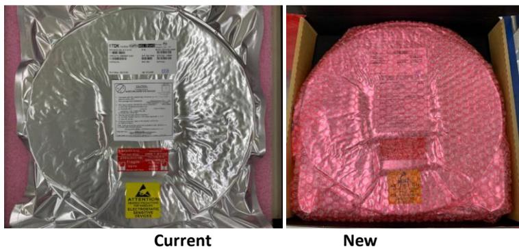
**Figure 29. Reel now packed for shipping in bubble wrap and pizza box**
