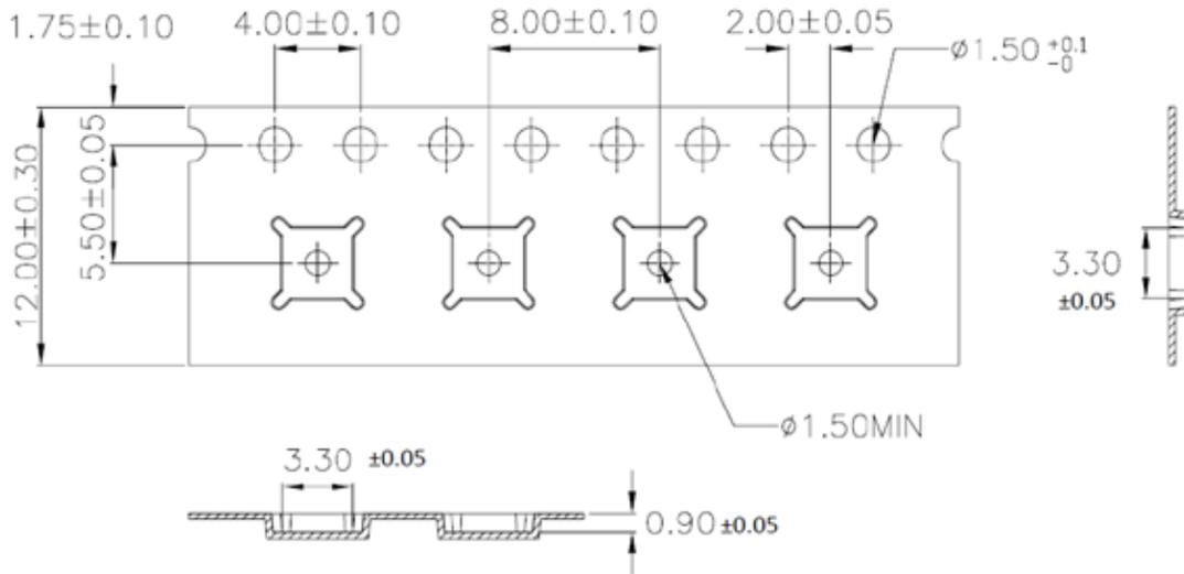
**Figure 17. 3 x 3 mm² Tape Dimensions (TYPE II) (for package height 0.75 mm)**
