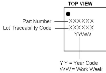
**Figure 14. 4.5 x 4.5 mm<sup>2</sup> QFN Package Marking Specification**
