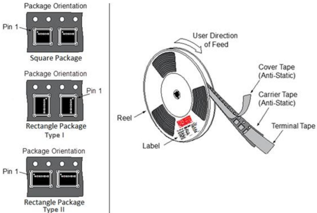
**Figure 23. Tape and Reel – Package Orientation**
