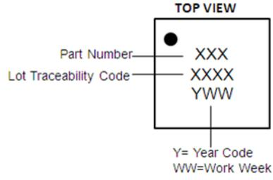
**Figure 12. 2.3 x 2.3 mm<sup>2</sup> Package Marking Specification**
