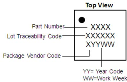
**Figure 9. 3 x 3 mm<sup>2</sup> Package Marking Specification (TYPE I)**
