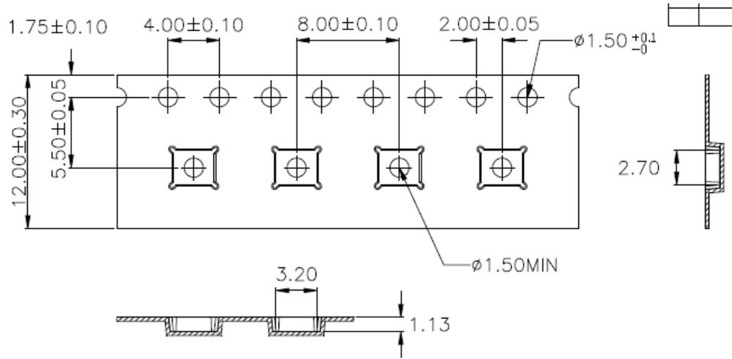
**Figure 20. 2.5 x 3 mm² Tape Dimensions (TYPE II) (for special request only)**
