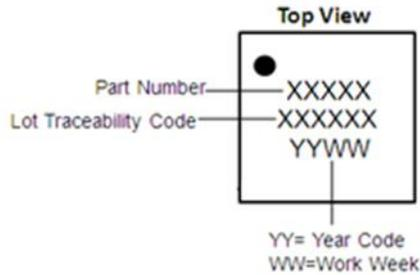
**Figure 10. 3 x 3 mm<sup>2</sup> Package Marking Specification (TYPE II)**
