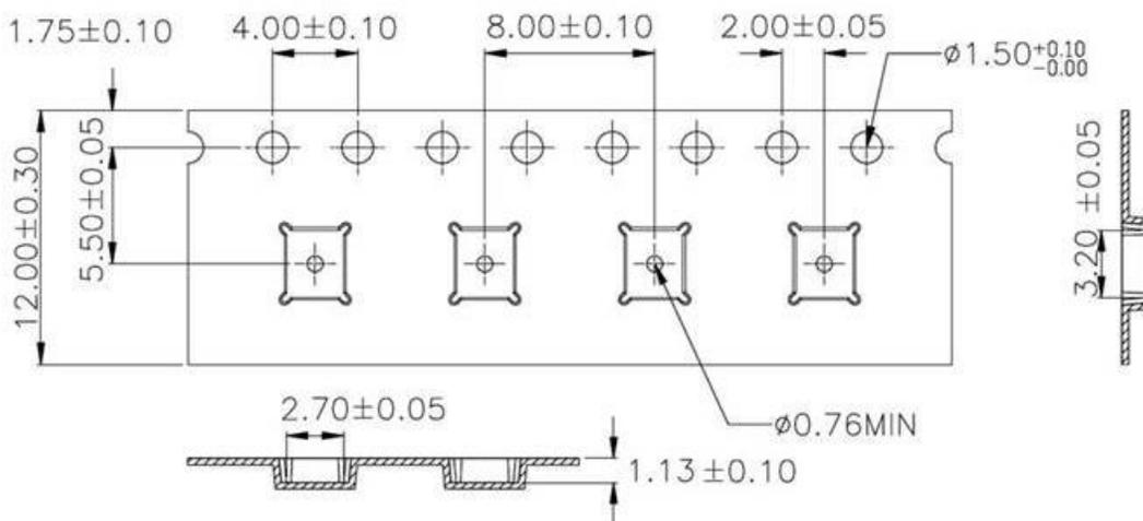
**Figure 19. 2.5 x 3 mm² Tape Dimensions (TYPE I)**
