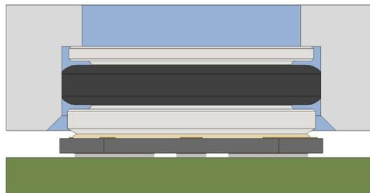
**Figure 8. Sensor with O-ring Sealed in Mechanical Housing**
