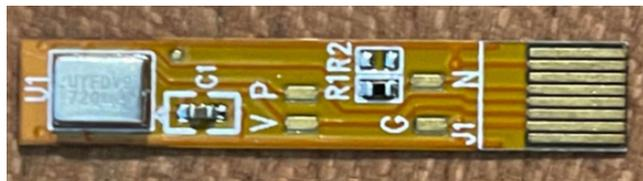
**Figure 3. Edge connector FPCB (Top side)**
