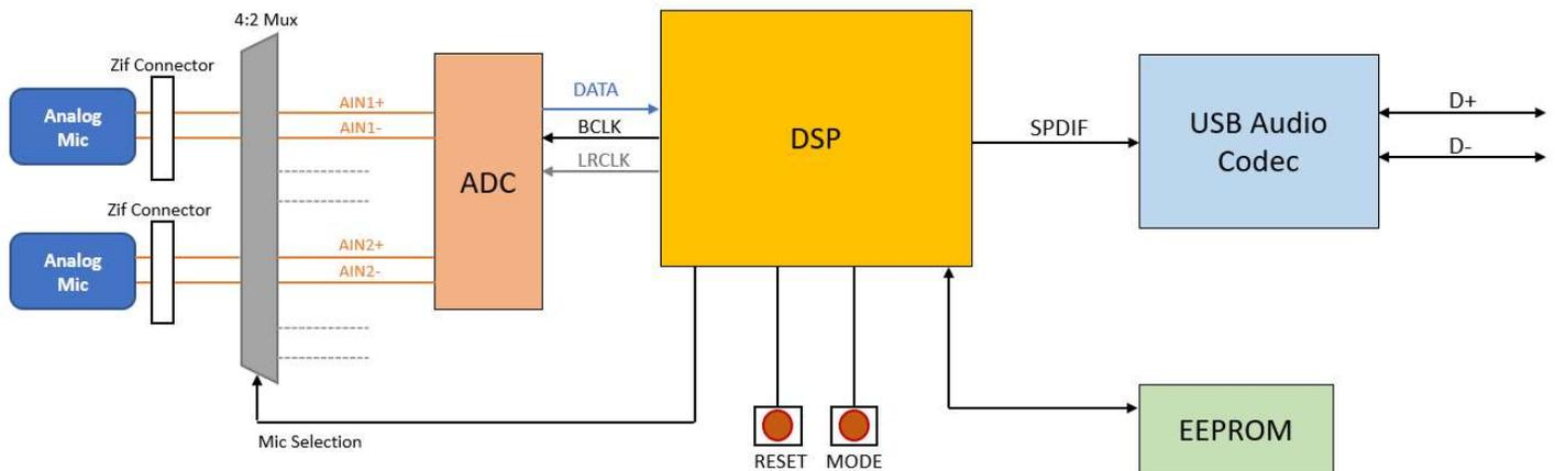
**Figure 10. Block diagram of analog signal path**
