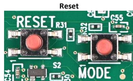
**Figure 7. Reset and Mode push buttons**
