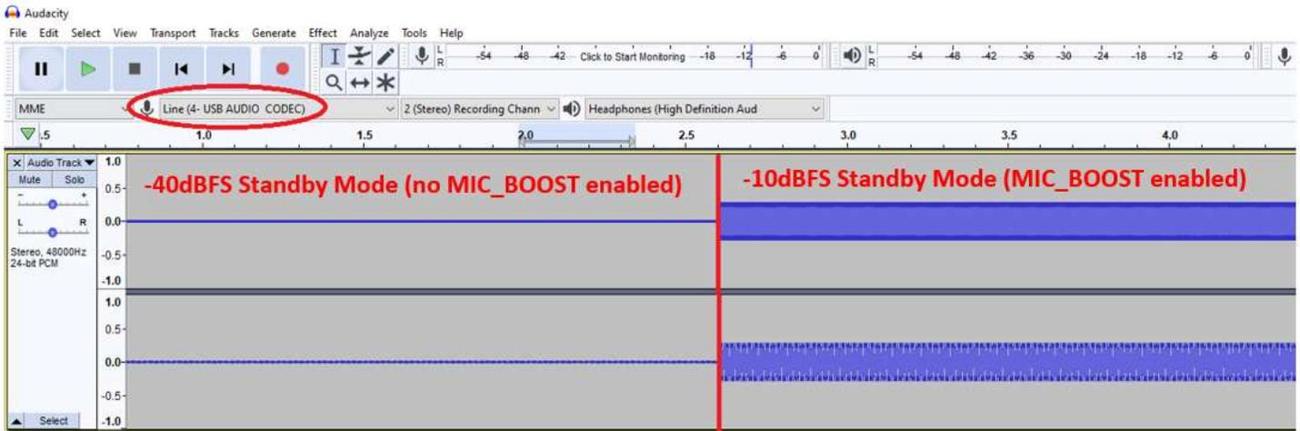
**Figure 6. Recording in Audacity – Standby mode test tones**
