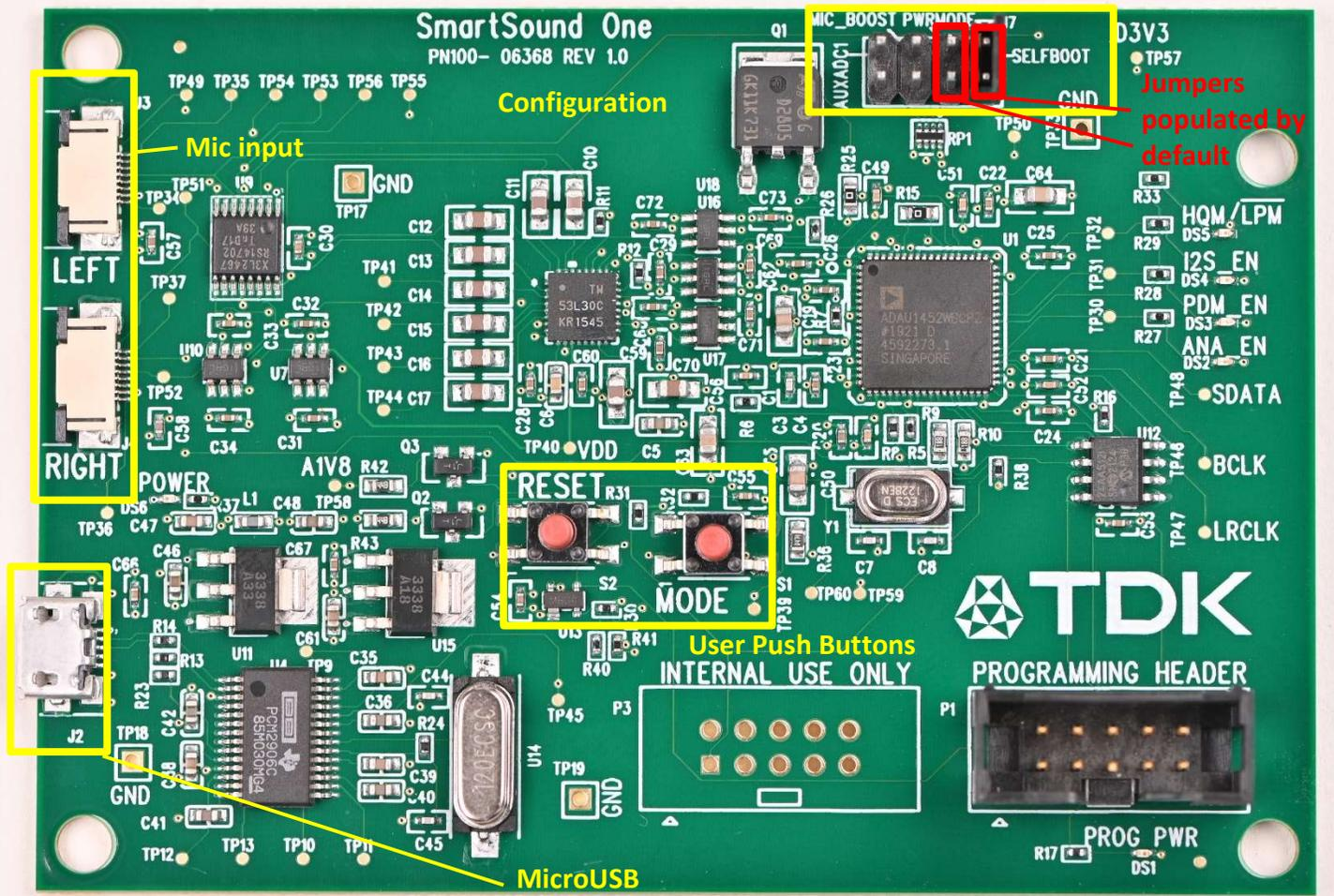
Figure 1. SmartSound One evaluation module with key components identified
