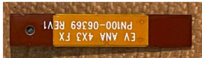
**Figure 4. Edge connector FPCB (Bottom side)**
