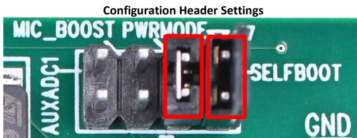
**Figure 9. Configuration header**
