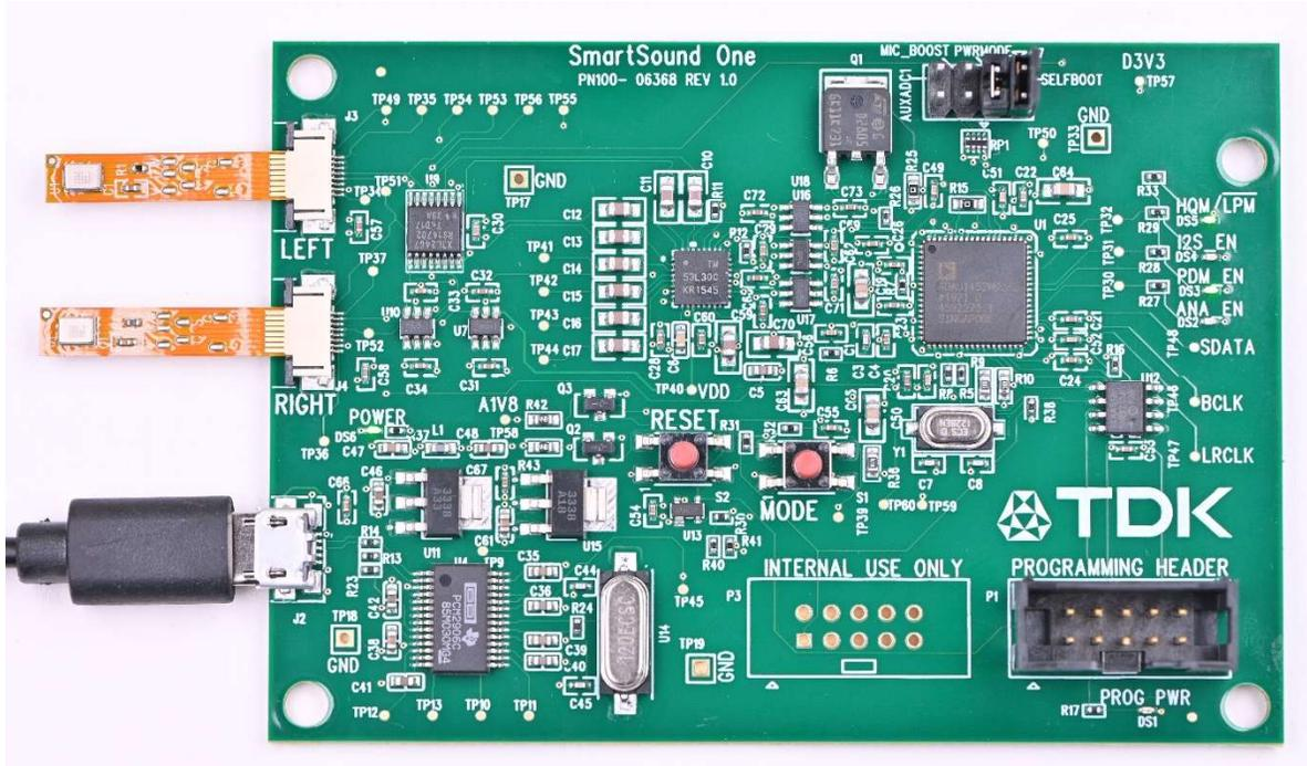
**Figure 2. Microphones connected to SmartSound One Module**
