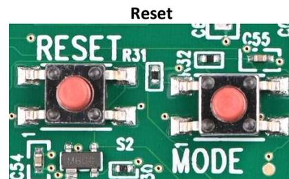
**Figure 7. Reset and Mode push buttons**
