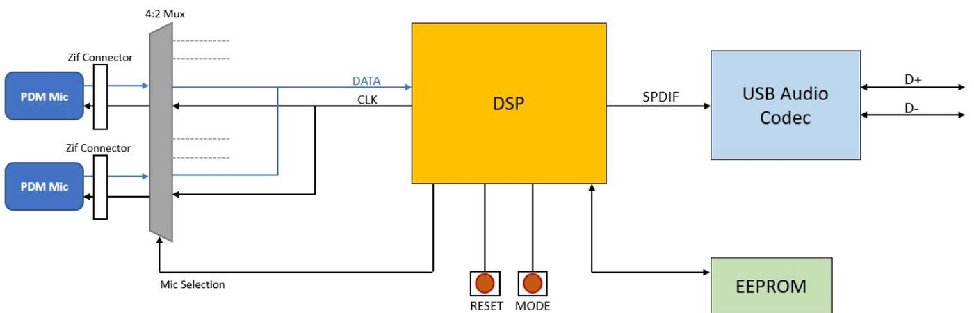
**Figure 11. Block diagram of PDM signal path**
