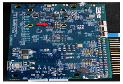
To connect in BLE mode switches 1&2 should be in OFF position, i.e. both downwards. Caution: Disconnect the USB power prior to modifying the DIP switch settings. The detailed procedure to connect USB or BLE is detailed in sections 6.2 and 6.3.
