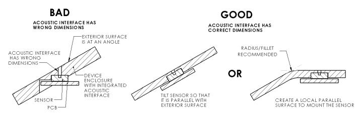
Figure 7. Cross-section views showing how to mount the sensor on an angled device enclosure surface.
