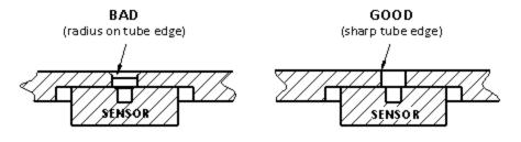
Figure 10. The exterior edge of a tube Acoustic Interface (highlighted blue) should be as sharp as possible to maintain a wide FoV.
