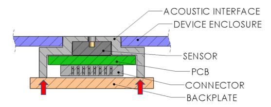
Figure 16. Example of a backplate-based module design to avoid applying excessive force on the sensor.
