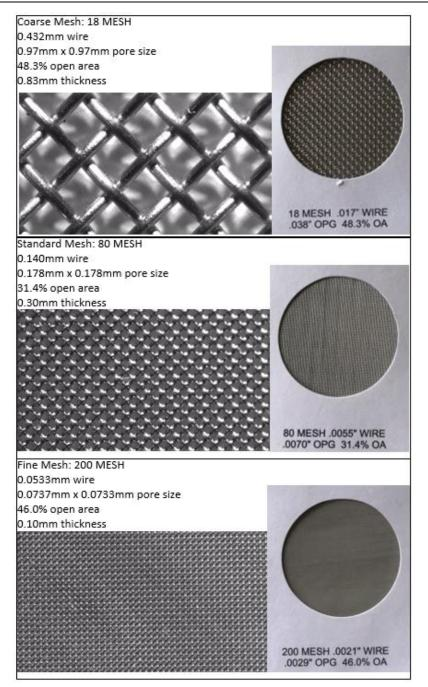
Figure 14. Examples of wire mesh materials.
