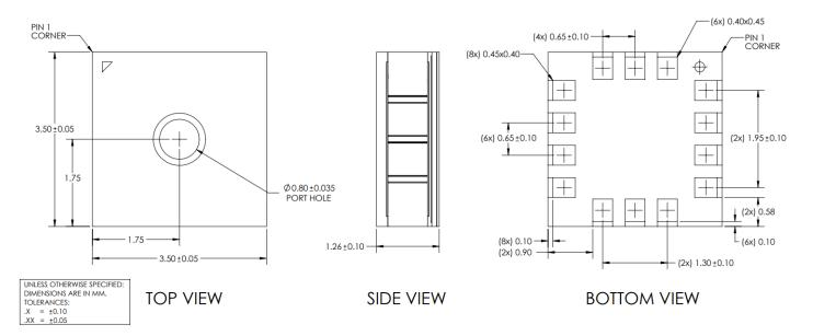
Figure 3. Package dimensions of the ICU-20201.
