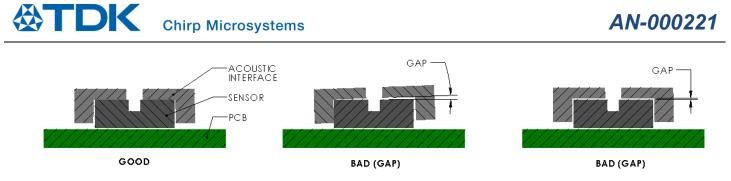
Figure 18. Examples of what good and bad assembly of the Acoustic Interface look like.
