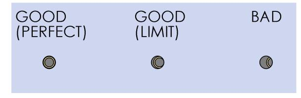
Figure 17. Examples of various degrees of sensor port alignment with the Acoustic Interface, from perfect concentric alignment (left), maximum acceptable limit tangent alignment (middle), to bad occluded alignment (right).
