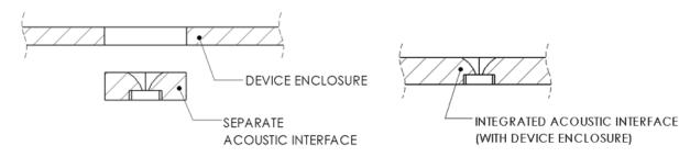
Figure 6. Separate Acoustic Interface (left) and integrated Acoustic Interface (right).
