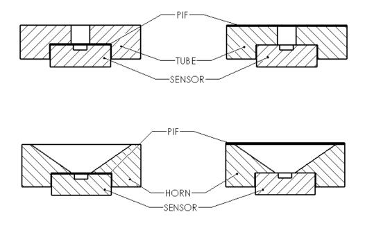
Figure 12. Examples of possible PIF placements for both tubes and horns.
