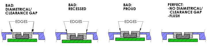
Figure 19. Bad assemblies create edges for ultrasound to reflect off from and affect the beam pattern.
