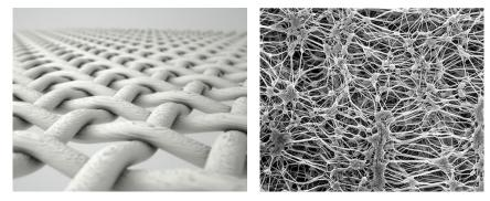
Figure 11. Representative close-up images of the structure of woven meshes (left) and nonwoven membranes (right).
