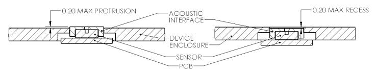
Figure 21. The Acoustic Interface should be mounted flush to the device enclosure to within 0.2 mm.
