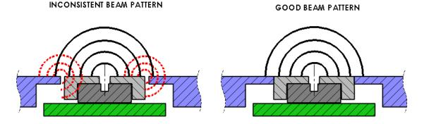
Figure 20. Effect of edges on the beam pattern.
