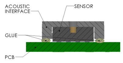
Figure 15. Cross-sectional picture showing where glue should be dispensed for attaching the Acoustic Interface.
