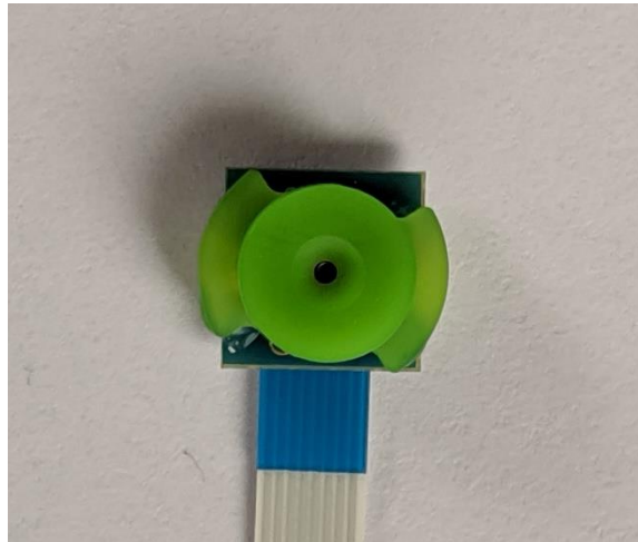
Figure 1. Chirp sensor module with acoustic horn
