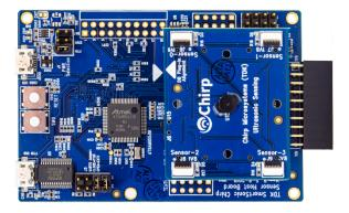
Part of the SmartSonic platform, the DK-CH101 is designed around Atmel's SAMG55 Cortex-M4 MCU and can be used by developers for rapid evaluation and development of CH101 based solutions. The DK-CH101 includes an on-board Embedded Debugger so external tools are not required to program or debug the SAMG55 MCU.
