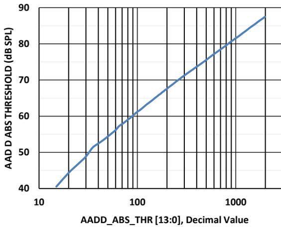
Figure 12. AAD Digital 1,2 Absolute Threshold vs Register Value
