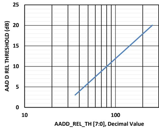
Figure 13. AAD Digital 1,2 Relative Threshold vs Register Value
