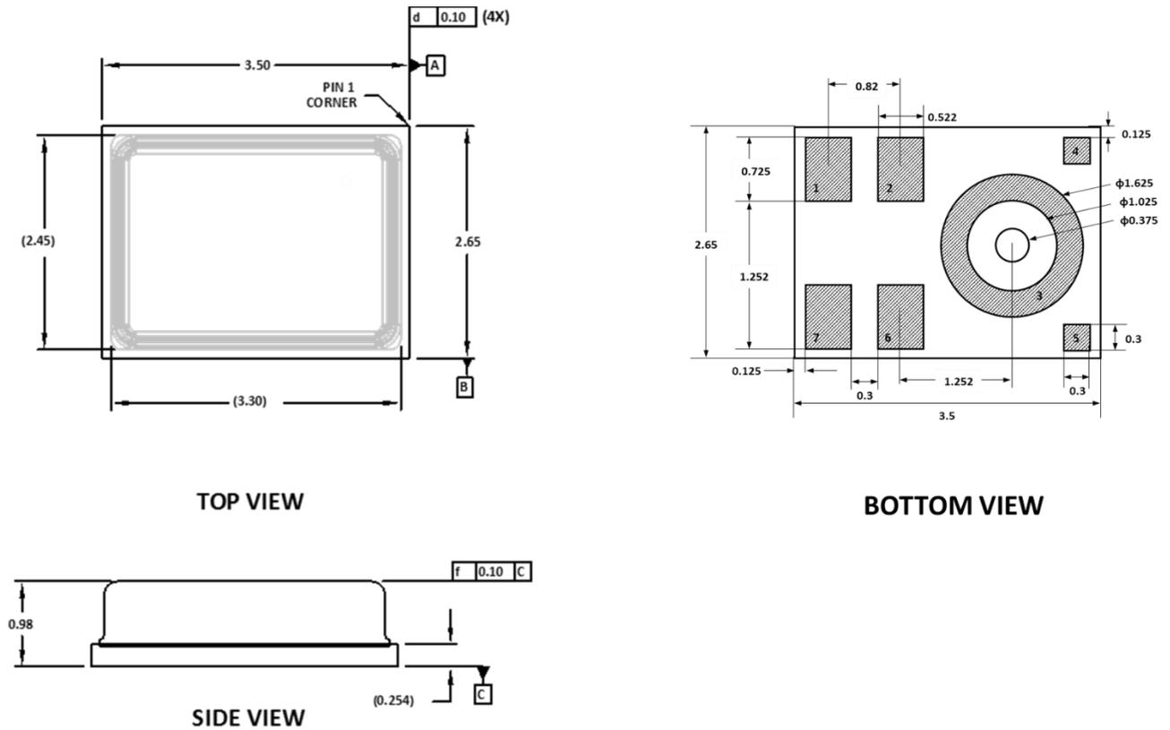
**Figure 34. 5-Terminal Chip Array Small Outline No Lead Cavity [LGA\_CAV]
