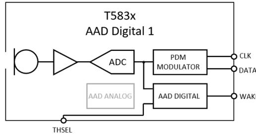
**Figure 17. Block Diagram for AAD Digital 1 Operation**
