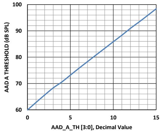
**Figure 11 AAD Analog Threshold vs Register Value**
