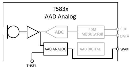
Figure 16. Block Diagram for AAD Analog Operation
