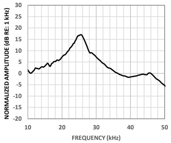
**Figure 9. Typical Ultrasonic Frequency Response, Ultrasonic Mode**
