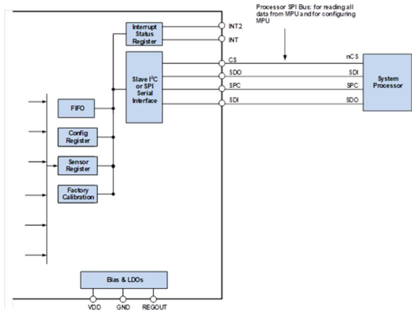
**Figure 7. IAM-20380HT Solution Using SPI Interface**
