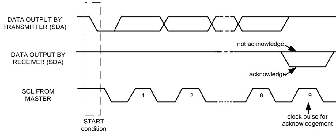
Figure 9. Acknowledge on the I<sup>2</sup>C Bus
