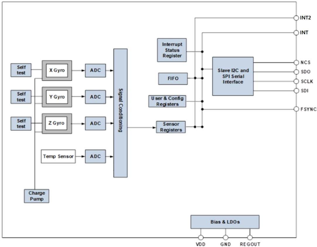
Figure 5. IAM-20380HT Block Diagram
