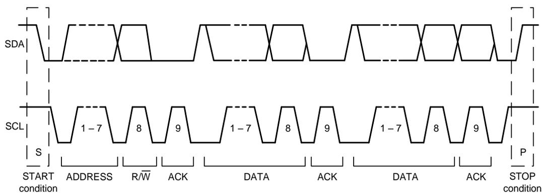
Figure 10. Complete I<sup>2</sup>C Data Transfer
