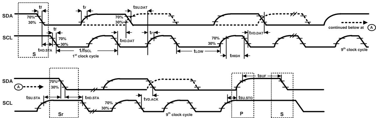
Figure 1. I<sup>2</sup>C Bus Timing Diagram
