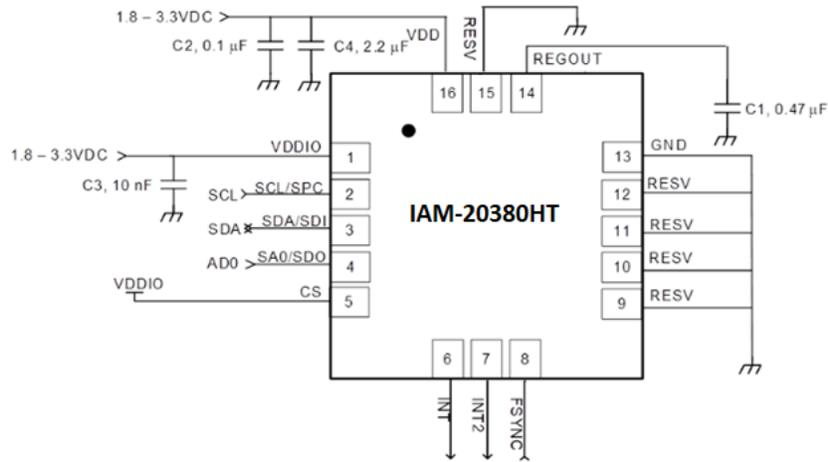
**Figure 4. IAM-20380HT LGA Application Schematic**
