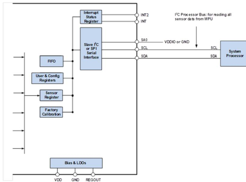
Figure 6. IAM-20380HT Solution Using I<sup>2</sup>C Interface
