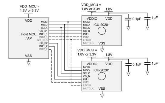
Figure 4. Multi-Transceiver Operation. Dashed connections are optional. Add additional transceivers by adding CS\_B and INT1 for each additional transceiver and sharing common MOSI/MISO/SCLK connections.
