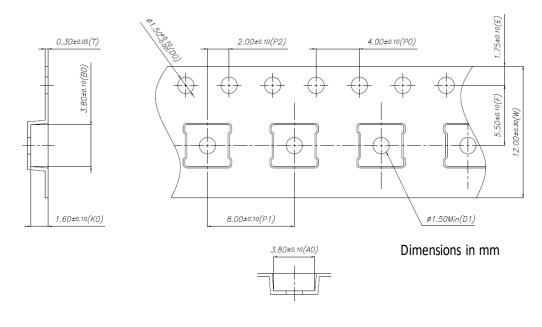
Figure 9. Tape & Reel Specifications
