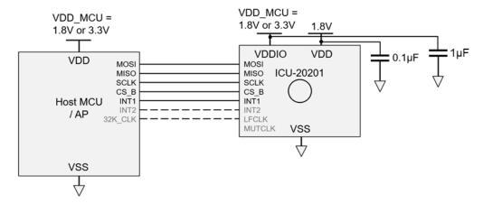
Figure 3. Single Transceiver Operation. Dashed connections are optional.
