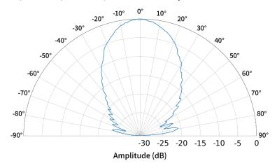
Figure 2. Typical Beam Pattern – MOD-ICU-20201-00-01 45 deg FoV module (Measured with a 1 m² flat plate target at a 1m range)
