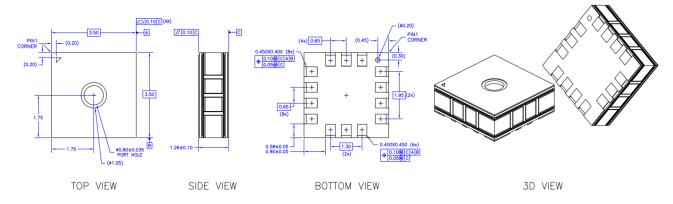
Note: All dimensions and tolerances conform to ANSI Y14.5M-1994.
