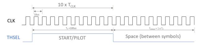
Figure 19. Timing diagram for example above showing relationship between THSEL pilot and CLK
