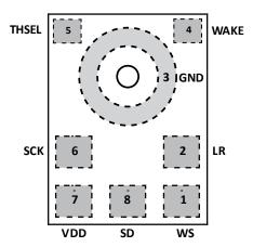
Figure 3. Pin Configuration (Top View, Terminal Side Down)
