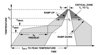
**Figure 2. Recommended Soldering Profile Limits**
