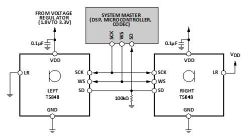
Figure 24. System Block Diagram
