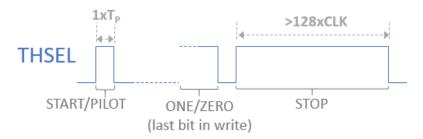
Figure 18. Write termination with Stop
