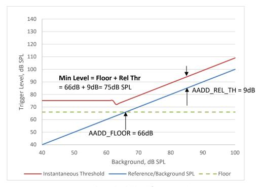
Figure 23. Relative Threshold with floor indicated
