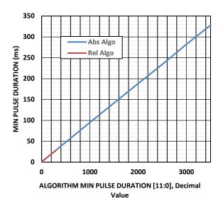
Figure 12. AAD Digital Min Pulse Duration vs Register Value
