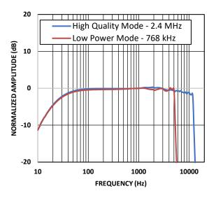
Figure 4. Typical Audio Frequency Response
