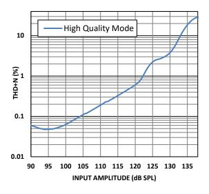
Figure 5. THD + N High Quality Mode – 1 kHz Input
