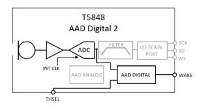
Figure 16. Block Diagram for AAD Digital 2 Operation
