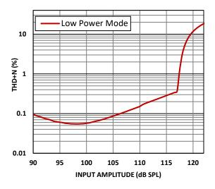
Figure 6. THD + N Low Power Mode - 1 kHz Input
