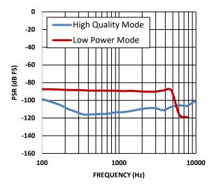
Figure 8. Power Supply Rejection (PSR) vs. Frequency
