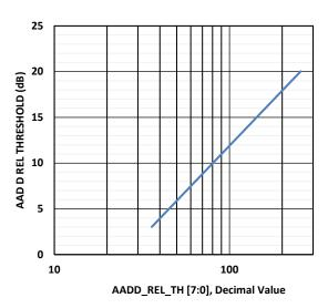
Figure 11. AAD Digital 1,2 Relative Threshold vs Register Value
