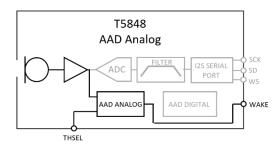
Figure 14. Block Diagram for AAD Analog Operation
