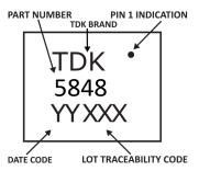
Figure 36. Package Marking Specification (Top View)
