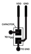
Figure 32. Recommended Power Supply Bypass Capacitor Layout
