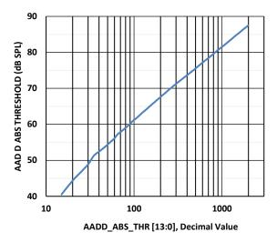
Figure 10. AAD Digital 1,2 Absolute Threshold vs Register Value
