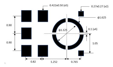
Figure 34. Suggested Solder Paste Stencil Pattern Layout
