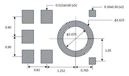
Figure 33. Recommended PCB Land Pattern Layout
