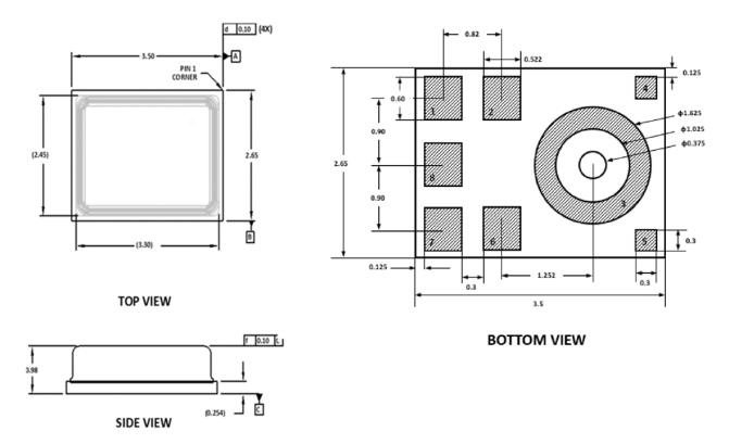
Figure 35. 8-Terminal Chip Array Small Outline No Lead Cavity [LGA\_CAV] 3.5 mm  $\times$  2.65 mm  $\times$  0.98 mm Body Dimensions shown in millimeters Dimension tolerance is  $\pm$ 0.15 mm unless otherwise specified
